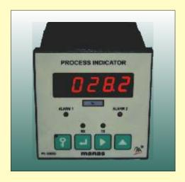
The PI - 100 D series is a compact sized Process Indicator, designed to accept input from any two wire or four wire Transmitter. It has a seven segment,  $\frac{1}{2}$ ", bright LED Display to read the Process Value in terms of Engineering Units or percent as is desired. The alarms can be set anywhere from 0% to 100 % with both High or both Low or one High and one Low configuration. The Output , 4-20 mA proportional to PV is isolated from input and power connections
